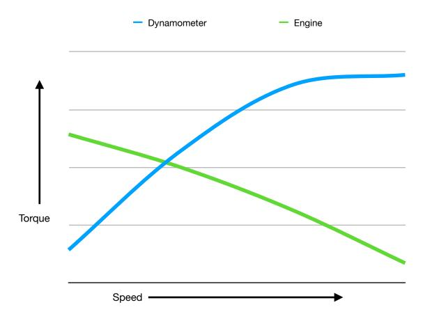
Therefore for every setting of the engine control (throttle) and dynamometer control there is a clearly defined torque/speed characteristic curve with a defined point of intersection.
