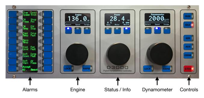
Some of the controls in these groups are fixed function and others have 'soft' functionality that can change if required. These adds to the flexibility of the D3000 controller and allows screens to change along with labels for functions.
